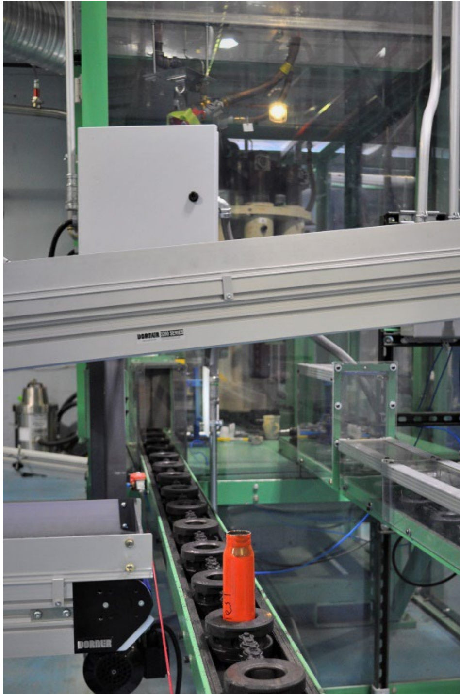
An empty 30-millimeter test casing prepares to enter the core of the Super Pull Apart Machine, or SPAM, during a briefing of the Crane Army Ammunition Activity machine's capabilities Feb. 20. (Photo by Randy Tisor)
